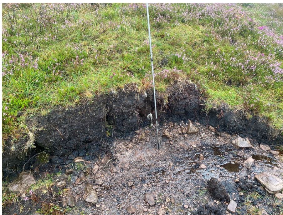
Plate 1 Typical profile - peaty topsoil layer over gravelly glacial till (Knocknanask)
